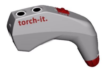
The Torch-it device uses ultrasonic waves to detect the presence of obstacles. These are sound waves which are not audible to human beings. The device has an ultrasonic sensor which can transmit as well as receive the ultrasonic waves. In the presence if obstacles are detected by the sensor of the device, if the obstacles from which waves are reflected lie within certain direction and distance range, a warning is issued to the user in the form of vibrations similar to a cell phone.
